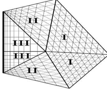
FIGURE 3. 2-d sketch of a possible meshing strategy near a singular edge. The thicker line represents the singular edge  $e_S$ .
