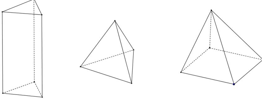
FIGURE 2. Meshes may contain triangular right prisms, tetrahedra or pyramids with parallelogram basis.
