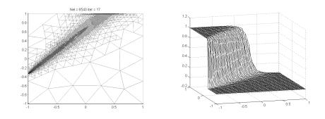
Fig. 4 Test 2, mesh and solution after 17 refinements.
